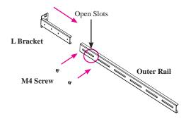
Secure L Bracket to outer rail with 1 or 2 M4 screws. Do not tighten yet.
